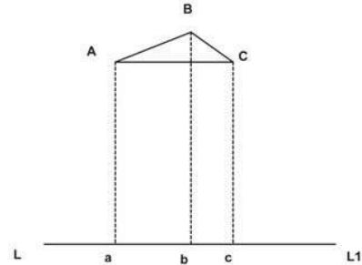
Figure 6.12 Orthogonal projection
