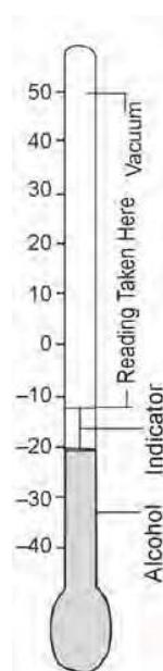
Figure 8.2 Minimum Thermometer
