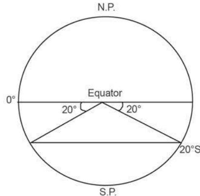
Figure 3.2 Drawing of Parallels of Latitudes
