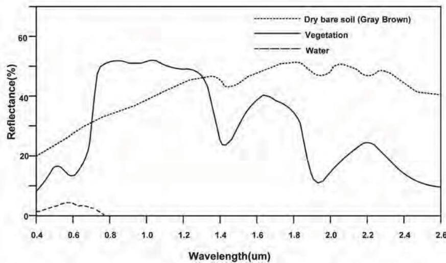
Figure 7.4 Spectral Signature of Soil, Vegetation and Water
