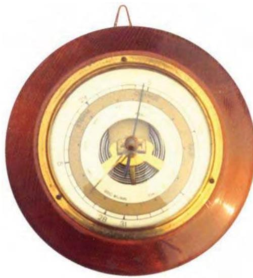
*Figure 8.5 Aneroid Barometer*
