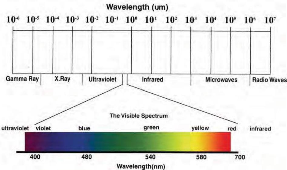
Figure 7.3 Electromagnetic Spectrum
