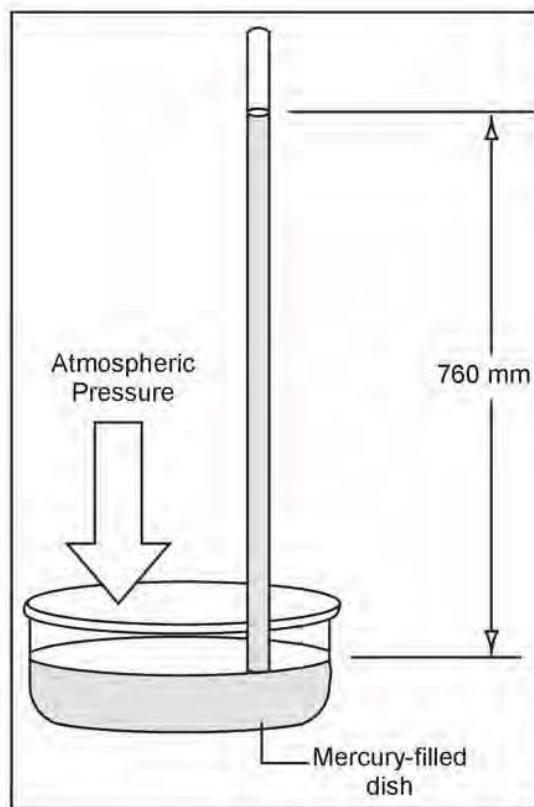
Figure 8.4 Mercury Barometer
