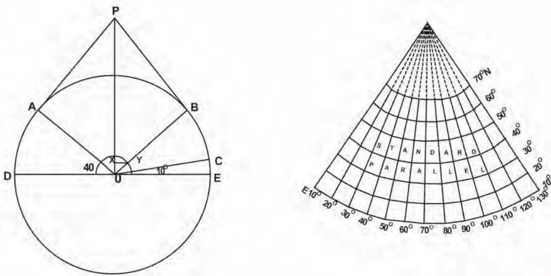
Figure 4.3 Simple Conical Projection with one standard parallel
