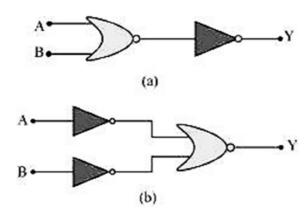
(A) A and B are the inputs and , is the output of the given circuit. The left half of the given figure acts as the NOR Gate, while the right half acts as the NOT Gate. This is shown in the following figure.
