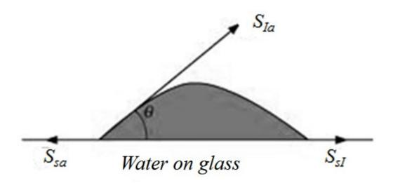
$S_{la}$ ,  $S_{sa}$ , and  $S_{sl}$  are the respective interfacial tensions between the liquid-air, solid-air, and solid-liquid interfaces. At the line of contact, the surface forces between the three media must be in equilibrium, i.e.,
