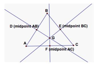
To find this point, you will construct three perpendicular bisectors, one for each side of the triangle. The point where all three perpendicular bisectors intersect is called the Circumcenter. Using this center point, we can draw a circle that passes through all three vertices.
