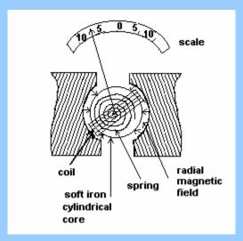
When the current is passed through the coil, a torque acts on it and is deflected. This deflection causes the restoring torque in the spiral springs attached at the two ends of the coil and the coil attains a steady deflection. The pointer attached to the coil moves on a scale and indicates the current.
