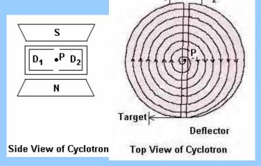
A positively charged particle is released at the centre P of the gap at time t=0. It gets attracted towards the Dee which is at a negative potential at that time. It enters the uniform magnetic field between the Dees perpendicularly and performs uniform circular motion in the gap. As there is no electric field inside the Dees, it moves on a circular path of radius depending upon its momentum and comes out of the Dee after completing a half circle.
