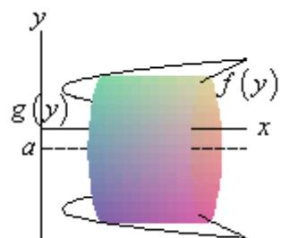
$$\begin{aligned} \text{radius:} & |a| + y \\ \text{width:} & f(y) - g(y) \end{aligned}$$
