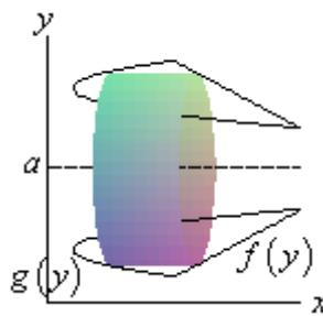
$$\begin{aligned} \text{radius:} & a - y \\ \text{width:} & f(y) - g(y) \end{aligned}$$
