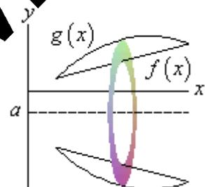
$$\begin{aligned} \text{outer radius:} & |a| + g(x) \\ \text{inner radius:} & |a| + f(x) \end{aligned}$$
