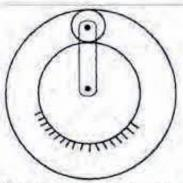
In the figure shown, the sun wheel has 48 teeth and the planet has 24 teeth. If the sun wheel is fixed, what is the angular velocity ratio between the internal wheel and arm?
