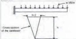
What is the ratio of the maximum compressive to the maximum tensile stress?
