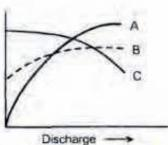
The above figure shows characteristics of three centrifugal pumps A, B and C. If E = Efficiency, H = Head and P = Power, the A, B and C respectively represent which one of the following 7
