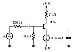
The small-signal voltage gain  $A_v = v_o/v_s$  is
